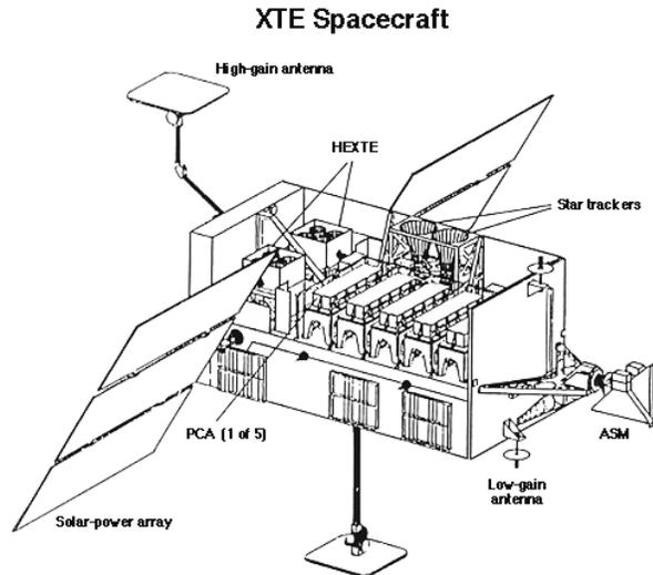
Figure 1.18: Schematic illustration of RXTE and all of its components. Source: NASA
