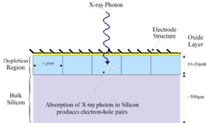
Figure 1.13: Simple diagram of a charge-coupled device. As X-ray photons enter the CCD depletion region electron-hole pairs are created. The electrons remain trapped in each pixel until they are read out. Upon this the position and energy of each incident photon is recorded.
