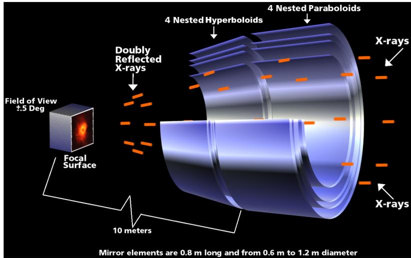
Figure 1.11: Schematic illustration of a the Wolter-I type mirrors composing the telescope on board Chandra observatory. Source: NASA/CXC/D. Berry 2010
