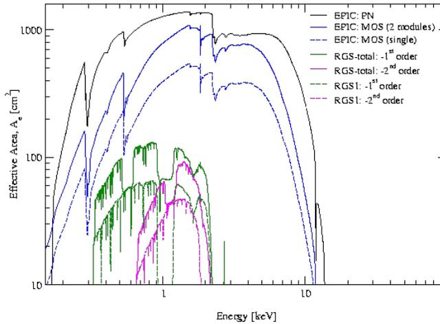
Figure 1.15: Effective area vs energy for all XMM-Newton detectors. Source: ESA
