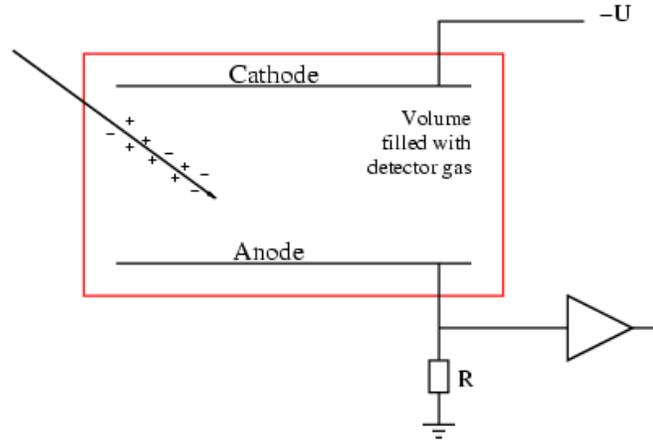
Figure 1.12: Simple diagram of a proportional counter. The space between the cathode and anode is filled with inert gas. Incident photons ionize the gas. Each event and its corresponding energy level is registered by the counter.
