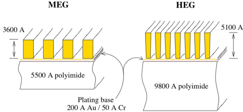
Figure 1.17: Schematic illustration of the cross-sections of the MEG and HEG membranes. All units are in Angstrom. Source: NASA
