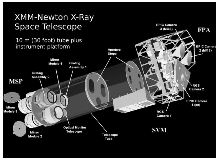
Figure 1.14: A schematic diagram of the XMM-Newton space observatory and its various parts. Source: ESA / AOES Medialab
