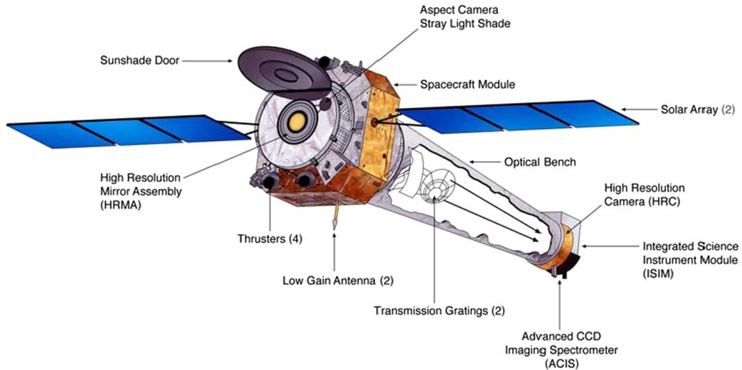
Figure 1.16: A schematic diagram of the Chandra space observatory and its various parts. Source: NASA
