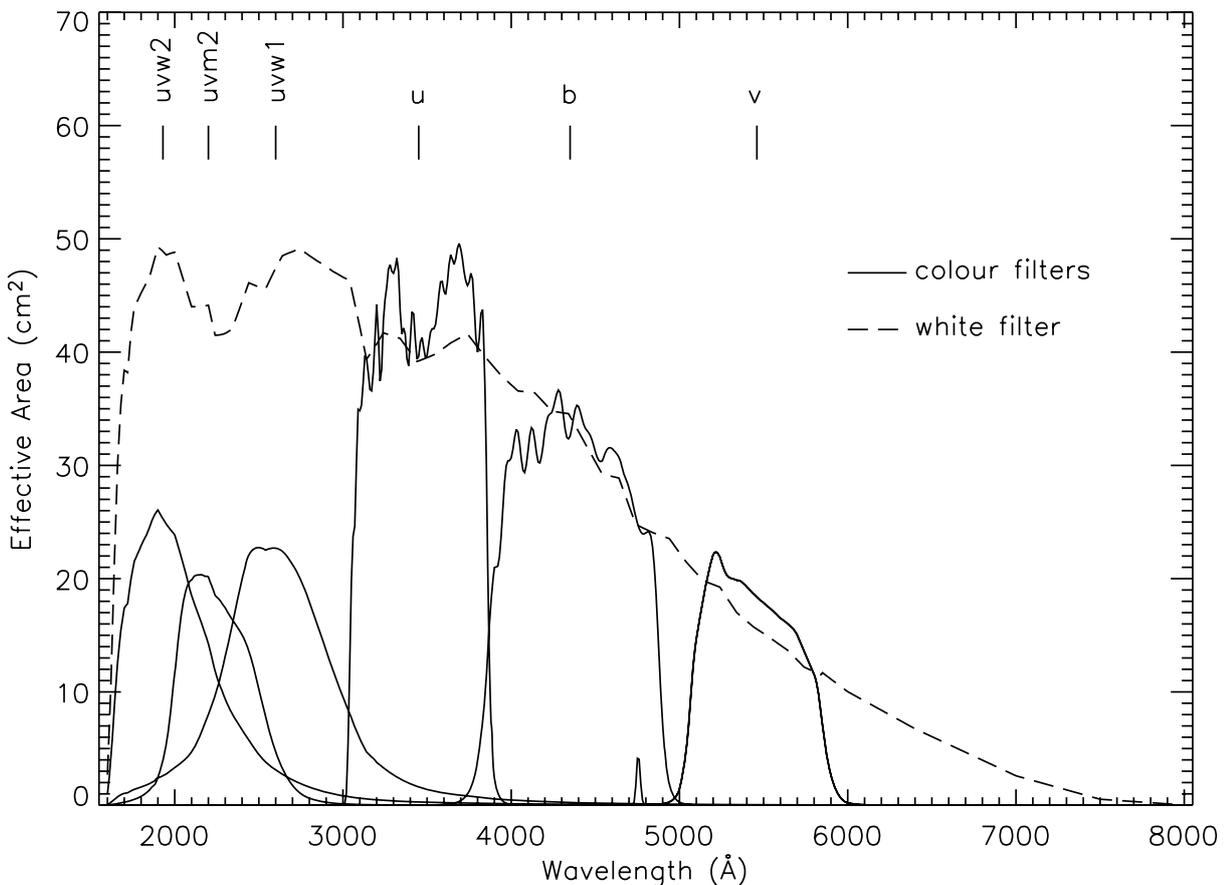
**Figure 2.1.** Effective-area curves for the seven UVOT filters. Graphics taken from Poole et al. (2008).
