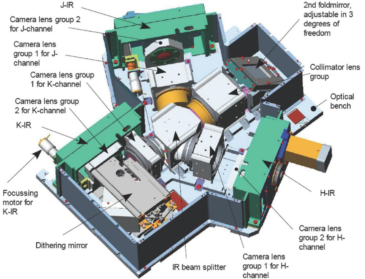
**Figure 2.3.** Infrared base plate with all optical and mechanical components. Apart from the splitters (see Fig. 2.2), the NIR arm is equipped with a focal reducer system, which consists of five collimator lenses and one camera lens for each NIR channel. This figure was taken from Greiner et al. (2008).
