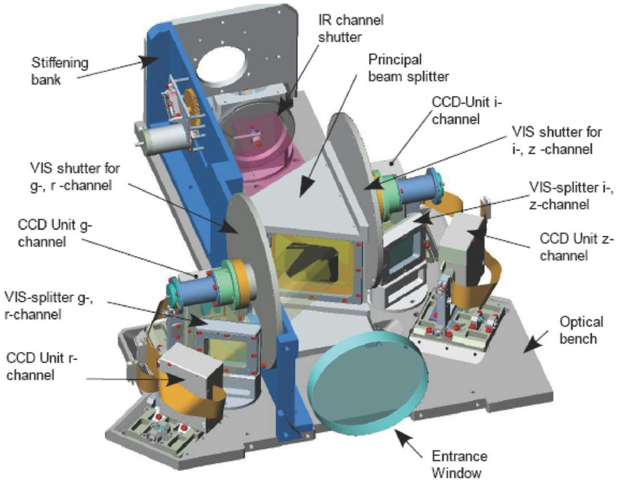
**Figure 2.2.** Visual base plate with nearly all optical and mechanical components marked. The splitters (or *dichroics* as in the main text) are defined by a certain wavelength value; radiation with longer wavelength goes through and the remainder with shorter wavelength is reflected. This figure was taken from Greiner et al. (2008).
