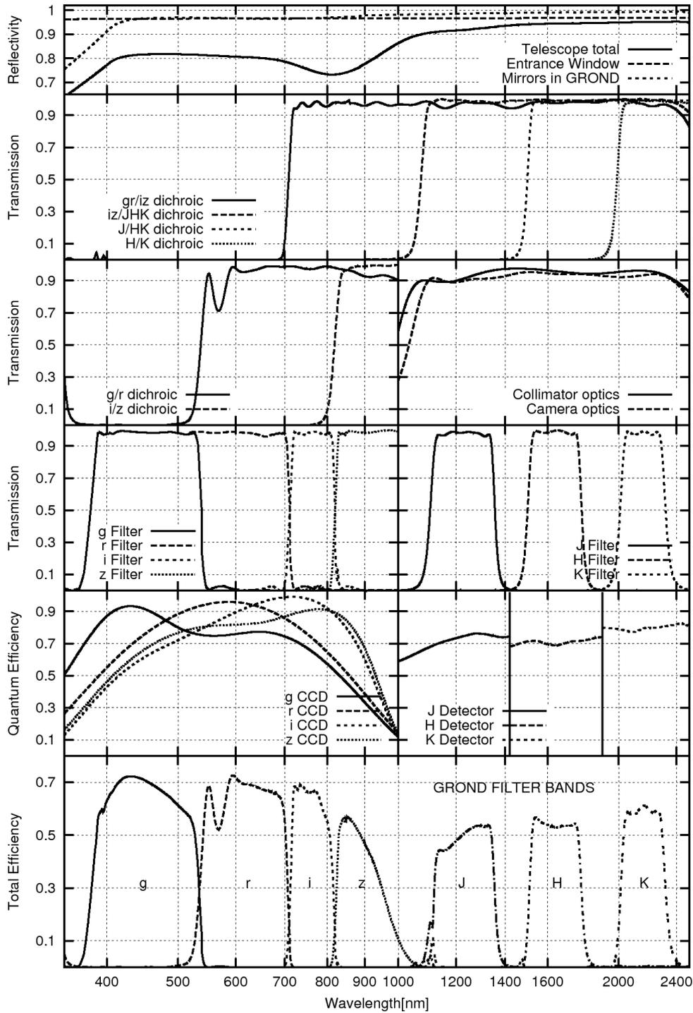
**Figure 2.4.** Efficiencies of the 2.2-m telescope and GROND along the light path. From the top, panels are: (1) reflectivity of the telescope and GROND-internal mirrors, (2) and (3) transmission of the dichroics and the NIR lens systems, (4) transmission of the filters, (5) detector quantum efficiency, and (6) the total efficiency in each of the seven GROND bands. This figure was taken from Greiner et al. (2008).
